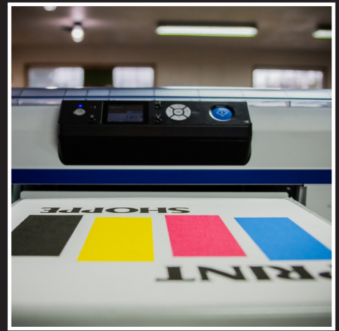
DIRECT TO GARMENT PRINTER USED TO PRINT FULL COLOR IMAGES ON FABRIC.
