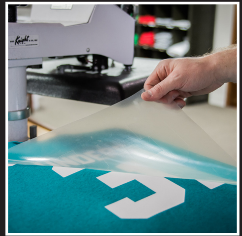
HEAT PRESS USED TO APPLY HEAT TRANSFER VINYL ON TO MATERIALS.
