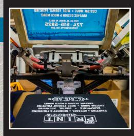
PRESS USED TO FORCE INK THROUGH SCREEN TO ON TO DESIRED SURFACE.
